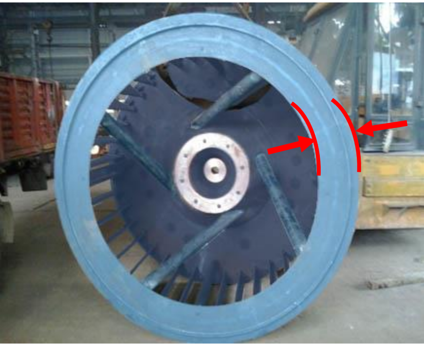
Introduced Hard faced liner to retard wear rate & for optimum sealing.
